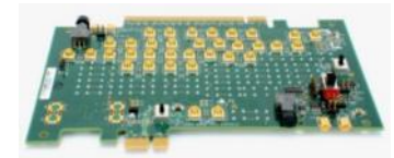
Load Board (System testing)
