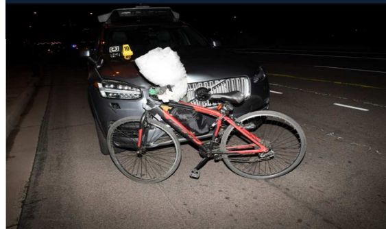
— A photo showing the bicycle matched up to the damaged area on the Uber Volvo. National Transportation Safety Board
