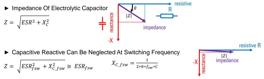
► ESR Can Be Calculated From Voltage And Current Switching Peak To Peak
