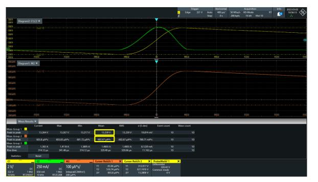
HD Mode with BW Limit 10kHz (16Bit)
