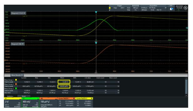
HD Mode With BW Limit 10kHz (16Bit) (Switching Frequency Rejection)
