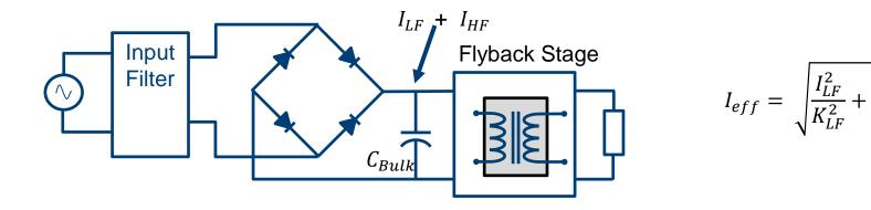
The Maximum Current Ripple Is Typically Defined At Line Frequency (100Hz)
