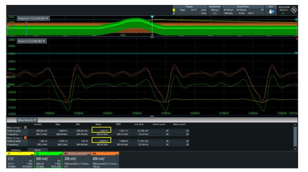
Results (@25°)  $U_{PP} = 1,02 V$  $I_{PP} = 1,85 \text{ A}$ ESR = 551 mO $F_{sw} = 285 \text{ kHz}$ Bandpassfilter (FIR)  $F_{stop1} = 13 \text{ kHz}$  $F_{pass1} = 125 \text{ kHz}$  $F_{pass2} = 11 \text{ MHz}$  $F_{stop2} = 11,25 \text{ MHz}$
