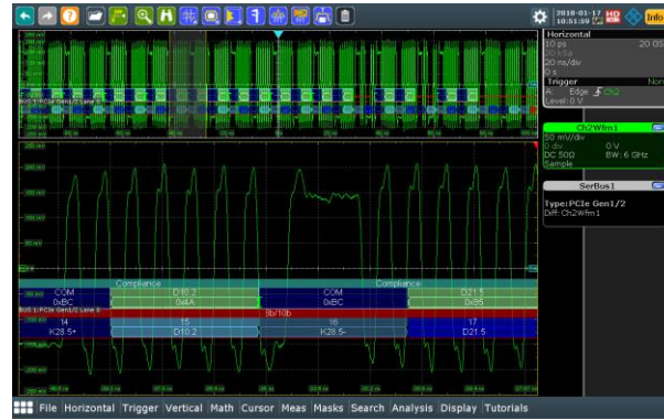
Decoding of 5 Gbps PCIe 2.0
