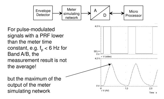
Example for pulse width = 10 ms, measurement time  $T_{meas} > 10 / f_p$
