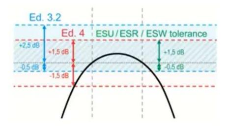
R&S® ESW, R&S® ESR and R&S® ESU are calibrated to a tolerance of -0.5dB/+1.5dB to comply with both CISPR 16-1-1:2004 (Ed.3.2) and CISPR 16-1-1:2015 (Ed.4) as common tolerance of both requirements.
