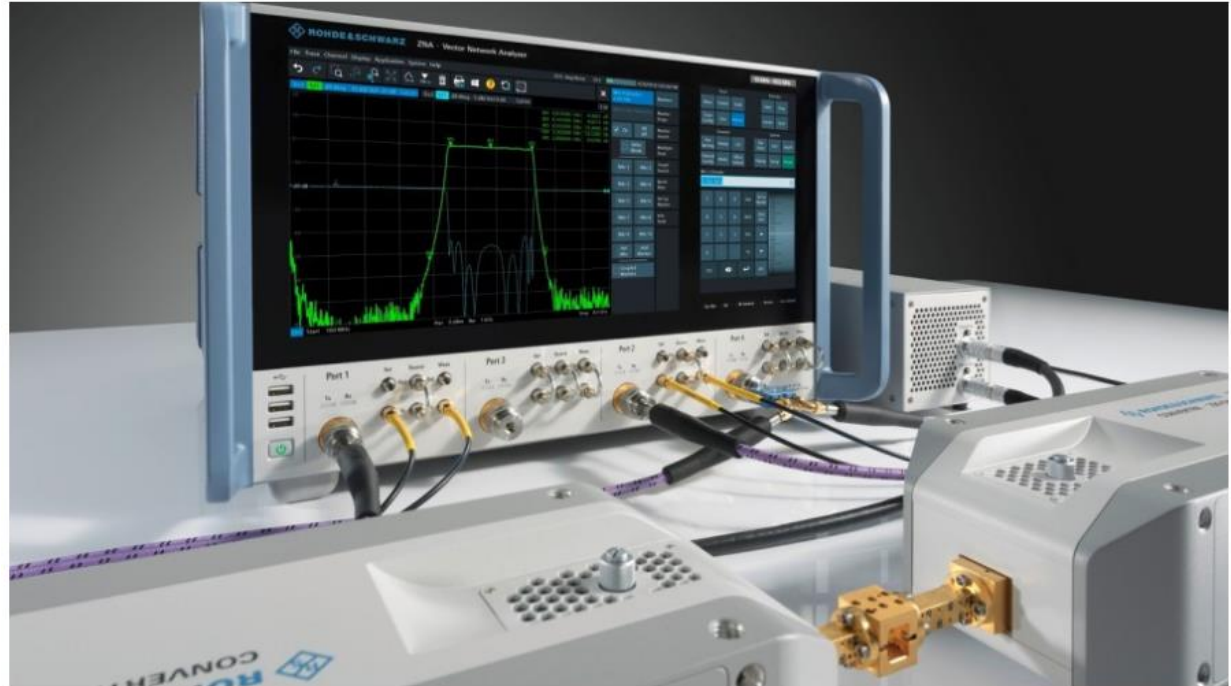
The R&S ZNA connected to R&S ZC170 frequency extenders allows S-parameter measurements in the D-band. (Image: Rohde & Schwarz)
