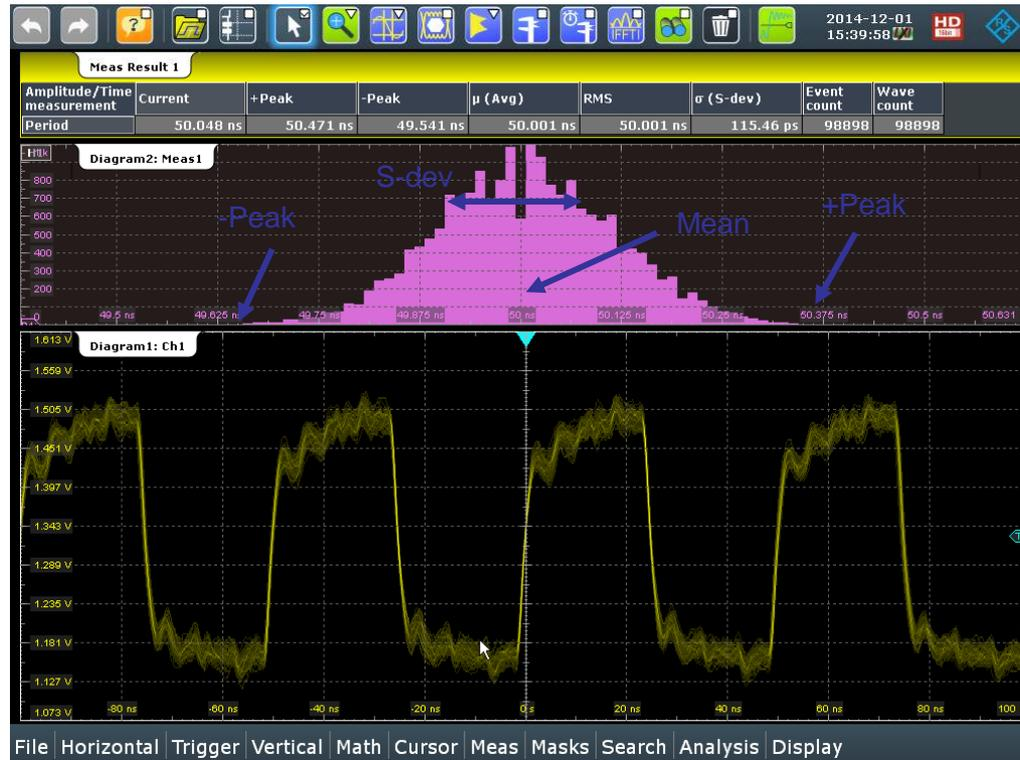
Peaks for unbounded jitter depends on measurement interval. Waveform count is important to limit the effect of such peak to peak jitter spread
