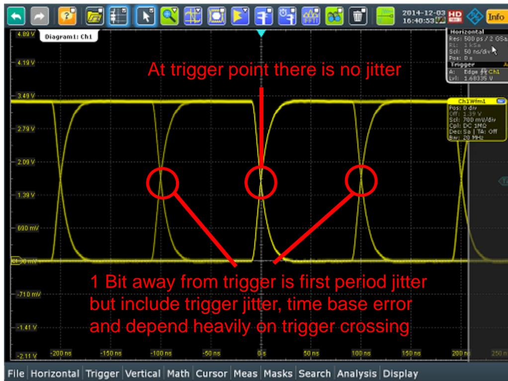
Not the best Eye Method because it is hard to determine if all transitions are overlap and jitter increase (time base error) as we move further away from trigger point.
