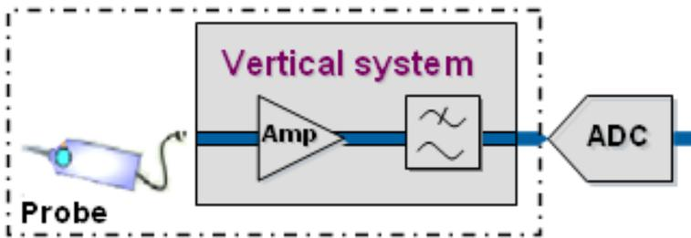
$$\left( \frac{1}{\text{BW}_{\text{system}}} \right) = \sqrt{\left( \frac{1}{\text{BW}_{\text{probe}}} \right)^2 + \left( \frac{1}{\text{BW}_{\text{scope}}} \right)^2}$$
