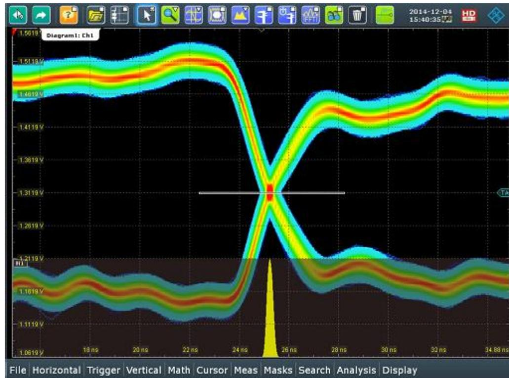
Histogram needs to be 1 pixel size around trigger value to see jitter distribution at the level
