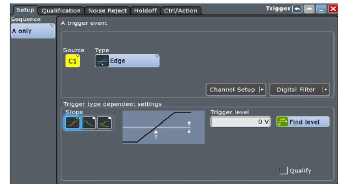
Trigger system basically work by aligning the position of all the samples that meet the required trigger condition relatively
