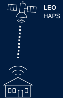
NR-NTN (VSAT, >10 GHz) Fixed wireless service with high gain ground antenna, terminals use VSAT/phased array
