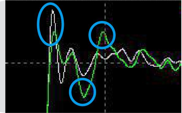
The impulse response of the probe is optimized with twisted test leads
