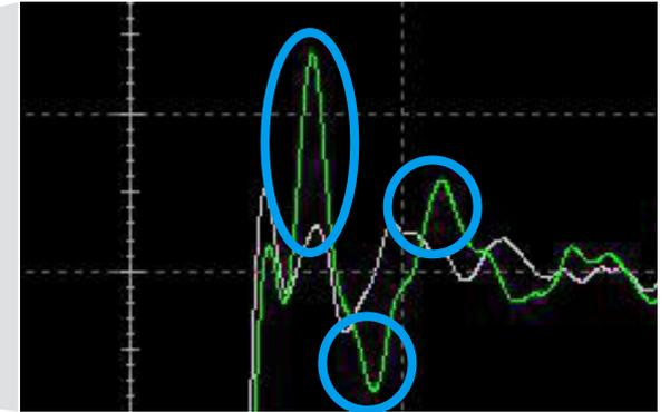
Clips have an influence on accuracy especially at full bandwidth (e.g. 200 MHz)
