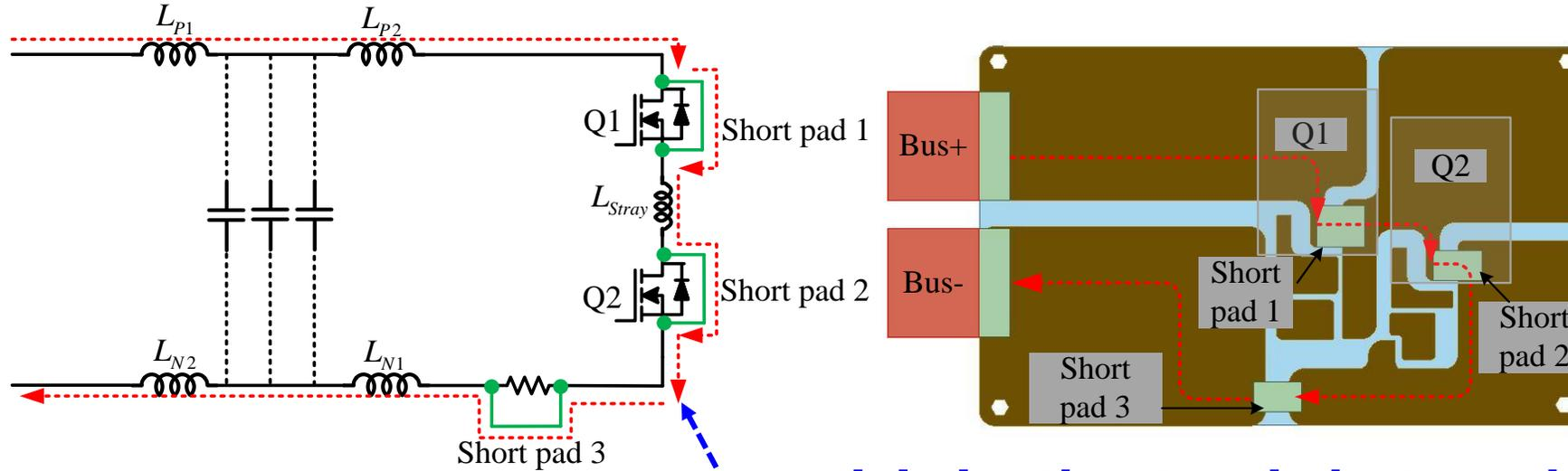
Minimize the stray inductance by Q3D to reduce turn-off voltage spike
