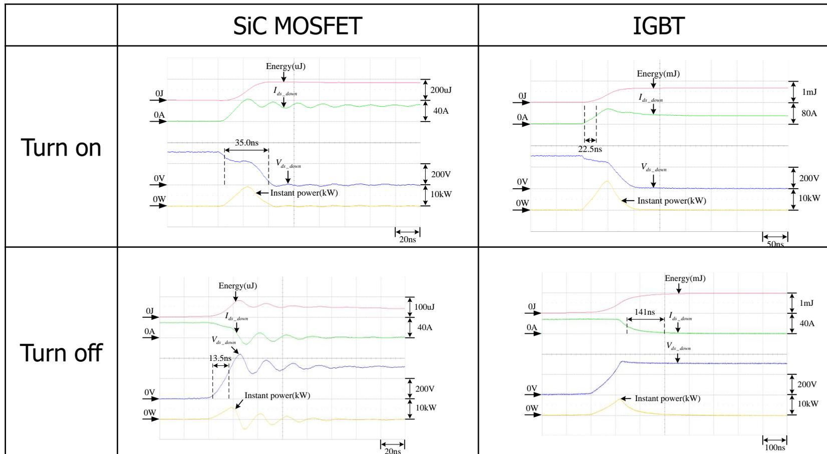
Switching loss of the SiC MOSFET and IGBT are 253.2 $\mu$ J and 1597.0 $\mu$ J, respectively.
