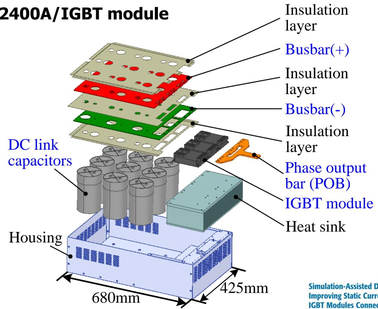
Simulation-Assisted Design of a Power Stack for Improving Static Current Sharing Among Three IGBT Modules Connected in Parallel
