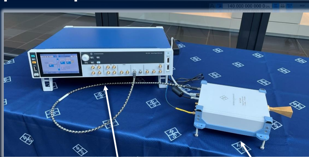
R&S®SFI100A Wideband IF Generator For modulation bandwidths up to 10 GHz
