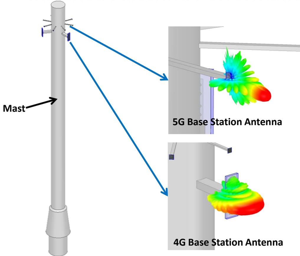
HFSS SBR+ simulation to calculate antenna pattern installed on a communication tower
