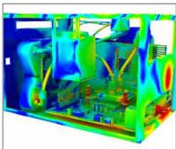
Simulates 3D electromagnetic fields to design high-frequency, high-speed electronic components. Its FEM, IE, asymptotic and hybrid solvers address RF, microwave, IC, PCB and EMI problems.
