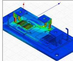
Calculates the parasitic parameter of frequency-dependent resistance, inductance, capacitance, and conductance (RLCG) for electronic products. Simulate and design electronic packaging and power electronic devices.
