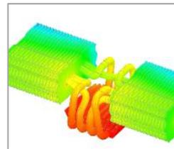
Predicts airflow, temperature and heat transfer in IC packages, PCBs, electronic assemblies/enclosures, power electronics. Icepak is a CFD solver for electronics thermal management.
