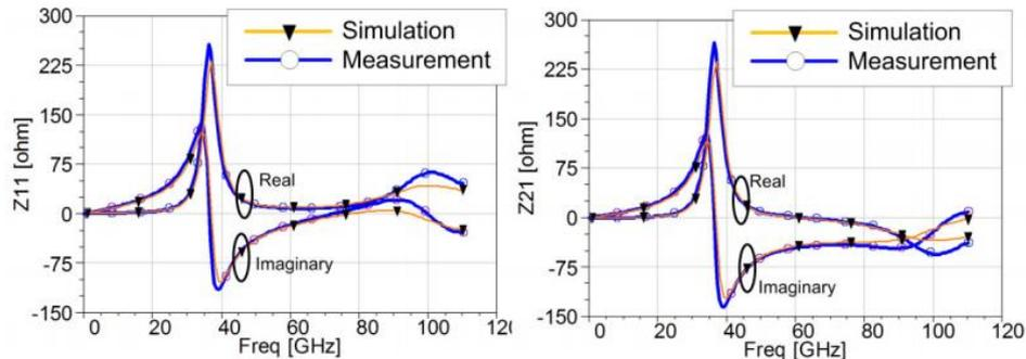
Figure 4. Measured and simulated Z parameters of the transformer
