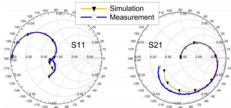
Figure 3. Measured and simulated S parameters of the transformer.
