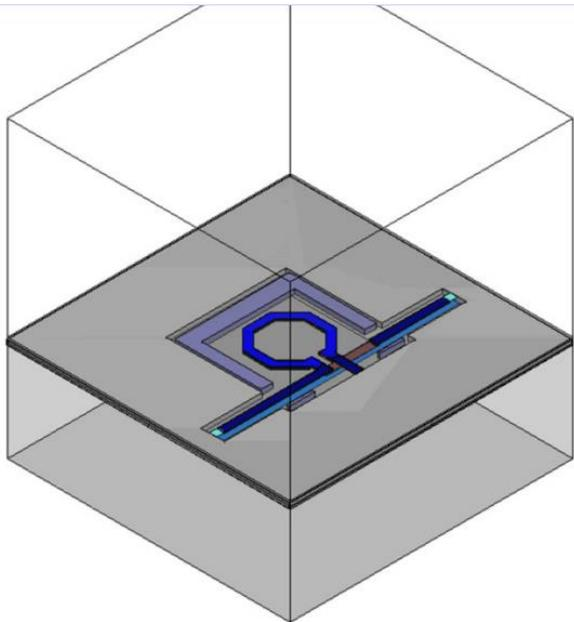
Figure 2. HFSS model of the transformer and interconnects.
