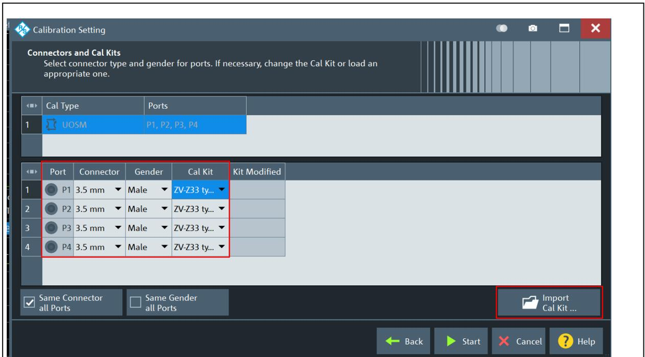
Figure3.1.1.11 設定 Connector & Gender & Cal kit
