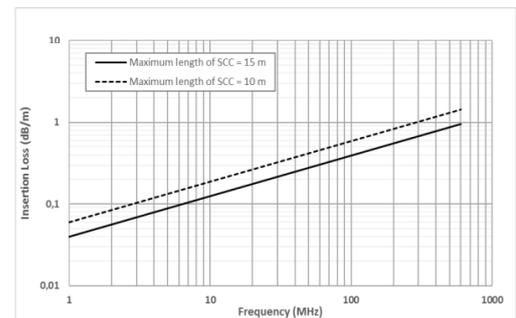
Figure 6.1.2-1: Insertion loss limit for cables
