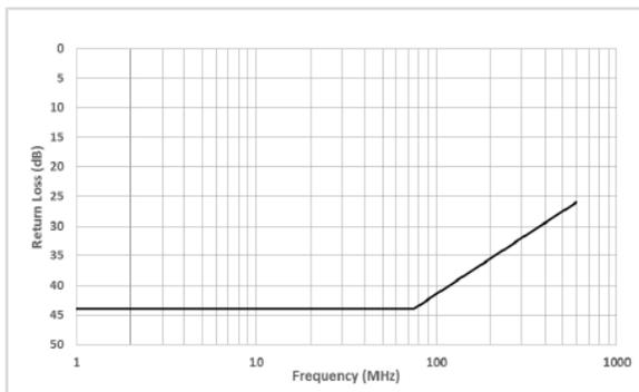
Figure 4.2-2: Return loss requirement for VNA calibration accuracy
