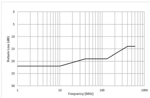
Figure 6.1.2-2: Return loss limit for cables
