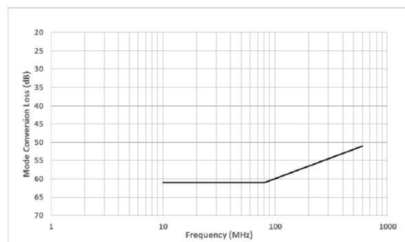
Figure 4.2-3: LCL / LCTL requirement for VNA calibration accuracy
