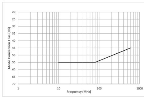
Figure 6.1.2-3: LCL / LCTL limit for cables
