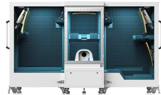
R&S®ATS1800M anechoic chamber
