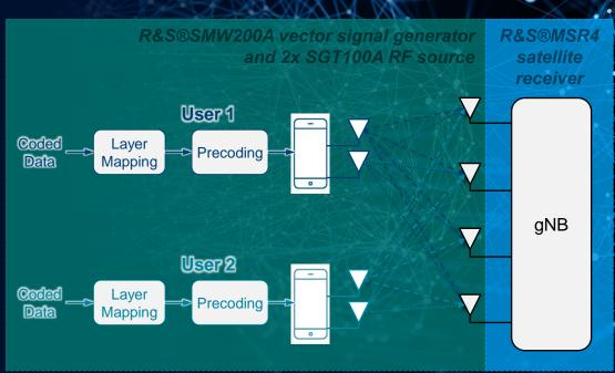
Both users transmit simultaneously on 80 MHz signal bandwidth (PRB 217), 16QAM modulation DMRS symbols 2 and 11, User#1 on even-numbered subcarriers, user#2 on odd-numbered subcarriers
