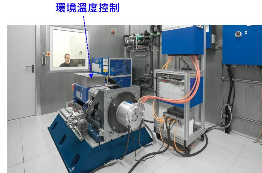
**Test bed for traction motor**
