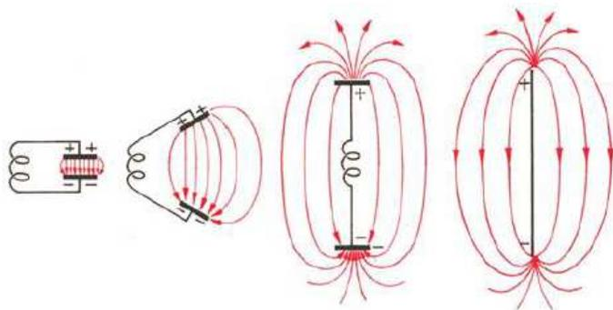
Figure 2: Heinrich Hertz's antenna model
