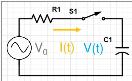
The higher the frequency, the lower the voltage, thus higher current. In general this means lower *impedance*.
