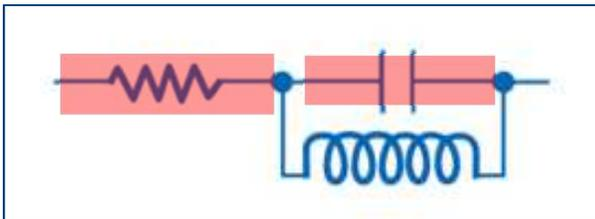
Inductor: includes capacitance of the coil and resistance of the wire
