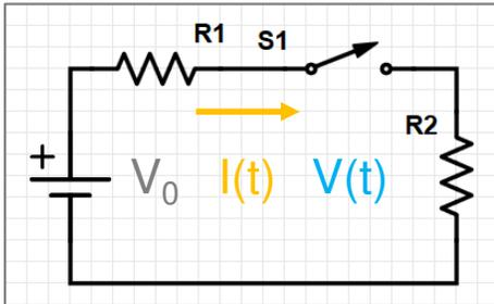
The current through a resistor is proportional to the voltage across it, and the voltage across it is proportional to the current through it
