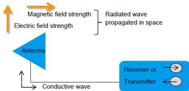
Figure 1: Basic antenna functionality
