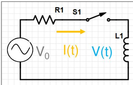
The higher the frequency, the lower the current. In general this means higher *impedance*.
