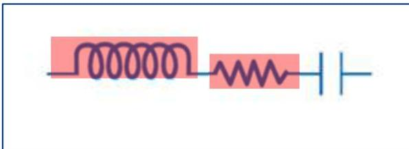
Capacitor: includes the lead inductance and series resistance
