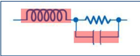
Resistor: includes capacitance of the structure and lead inductance
