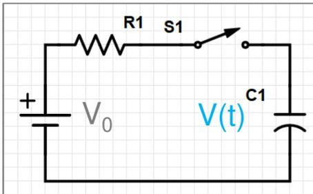
Capacitors resist any instantaneous changes in voltage.
