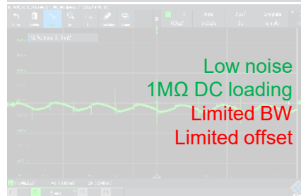
Low BW 1:1 passive probe
