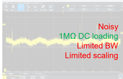
Standard 10:1 passive probe
